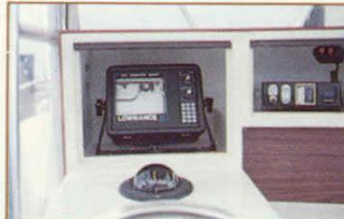
Lockable chart-recorder box with plexiglass shield removed
