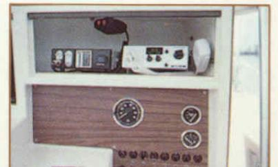
Lockable, radio box with plexiglass shield removed
