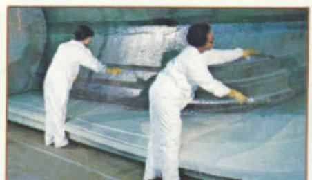
3. Hand-laid fiberglass mat and woven roving means a stronger, safer hull and deck. The hand lay-up process gives control of the fiberglass-to-resin ratio, insuring the uniform strength we require.
