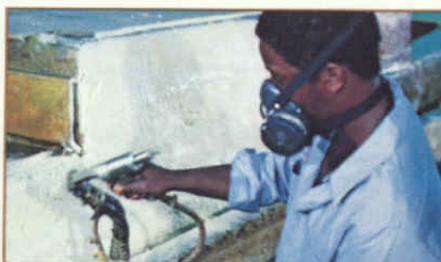
5. Strategic cavities in the hull and deck are filled with polyurethane spray which adds floatation, sound absorption, thermal insulation and hull strength.
