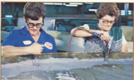
7. Every piece of standard hardware is through-bolted with locking nuts for long-lasting strength and safety.
