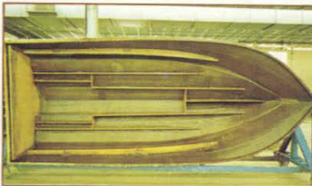
4. Stringers are encapsulated in resin and fiberglass and glassed into place while the hull cures in its mold. This gives your hull permanent strength and shape.
