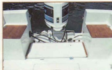
Fold-down motor well bulkhead (down)
