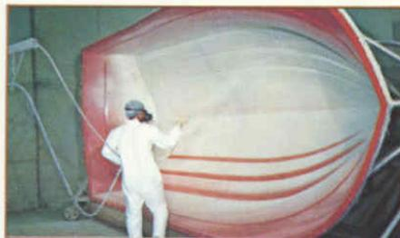
2. The finest NPG gelcoat is applied in our dust-free spray booths giving a smooth, durable finish to the hull and deck.
