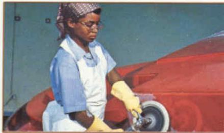
1. The mold determines the boat's shape and finish, so we carefully inspect each one, then polish it to insure a smooth finish.
